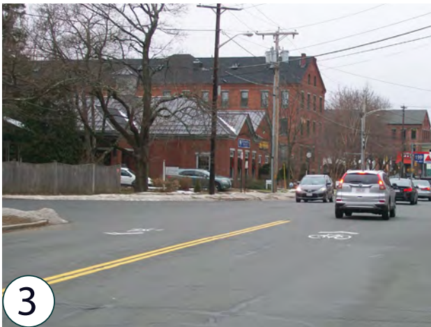
3 Extremely large turning radius to S Main St from Main St. (aA upper left portion of photo.)
