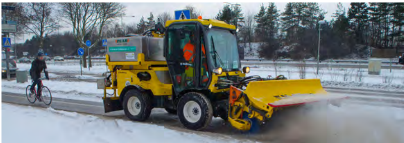
Specialized snow removal equipment in Sweden are designed for operation in separated and protected bike lanes.
