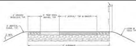
**6' WIDE ASPHALT WITH 3' WIDE TRAP ROCK GRAVEL**
